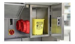
**Solid waste compartment\*** - The waste is stored in the compartment through an opening on the work surface. The waste is then removed through the shielded front door. This process follows the GMP guidelines, according to which, the waste must not be removed directly from the sterile work area.
